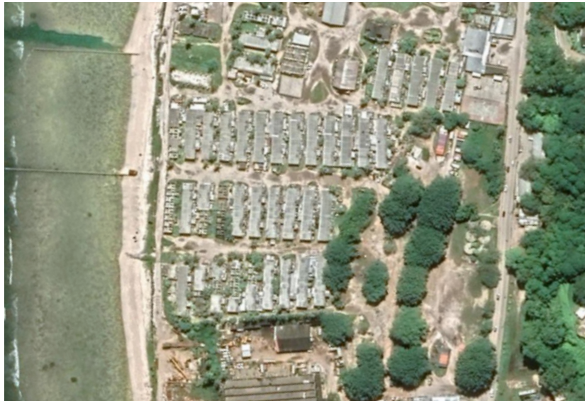
The British Phosphate corporation built this housing for ex pat workers prior to Nauruan independence in 1968. The uniform buildings, sited in long rows, are 25 feet wide with 25 feet between them. The buildings are all about 140 feet long. Where the second floor units have collapsed many ground floor units remain occupied. One photo shows how close the housing comes to the water and where it is in relationship to the ships that take phosphate from the port. Top left and bottom left photos taken by Vlad Sokbin, https://roadsandkingdoms.com/2015/no-way-nauru/
