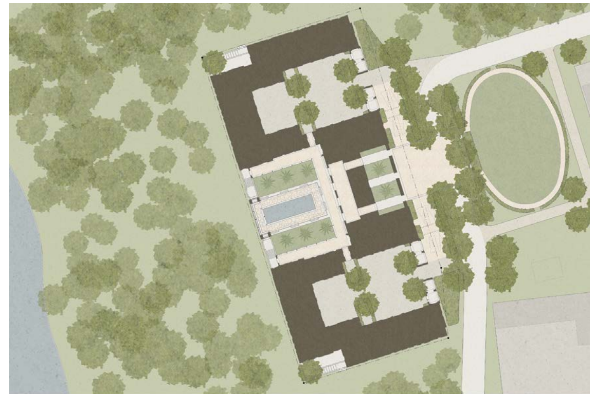
Above Right: A speculative site plan showing how a mirrored plan would work on a large 330 foot block with auto court access off an alley. Below Right: Site plan of the one acre site.
