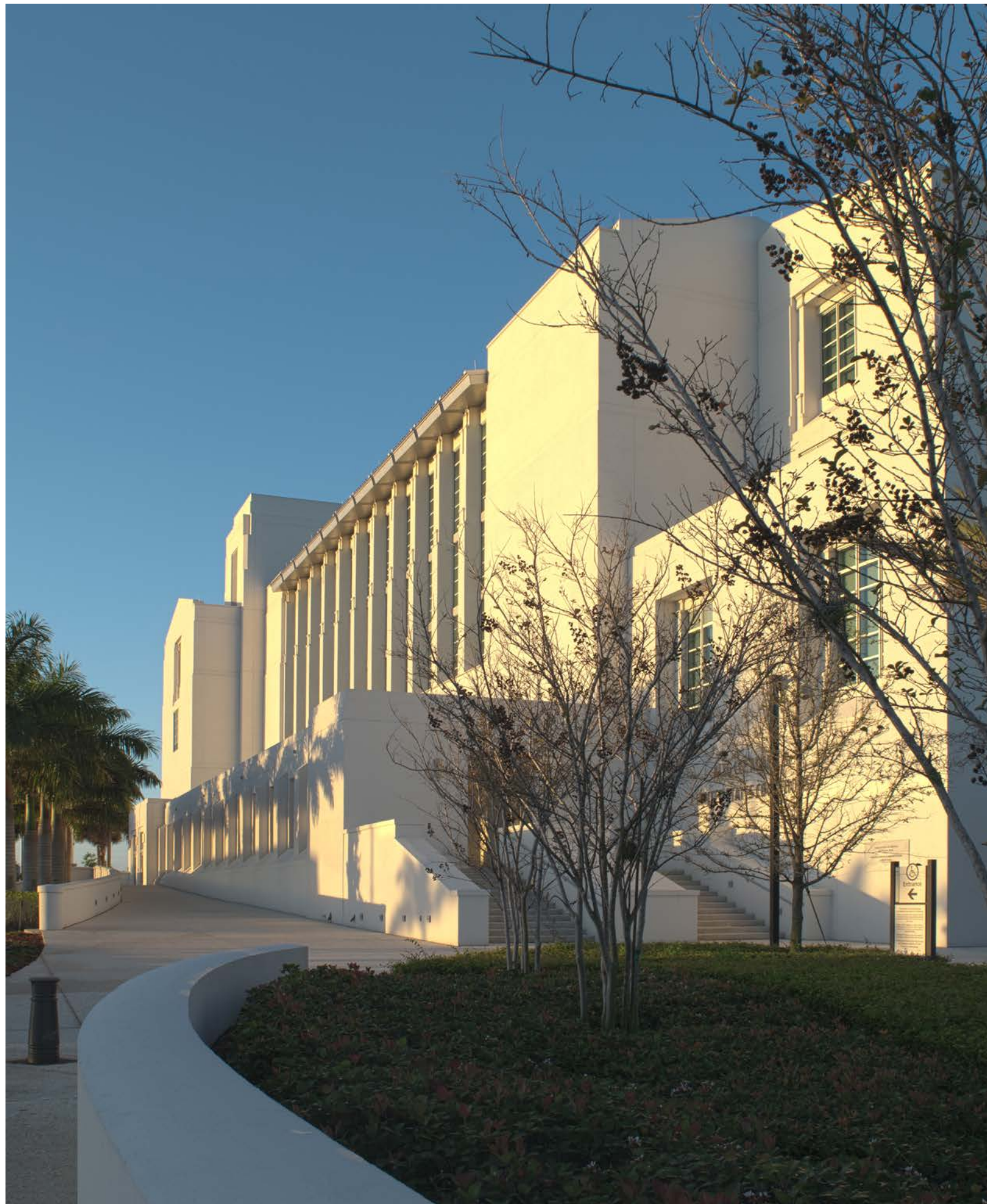
There is a high water table, and the parking level pushes the main floor a full level above the street. There are three ways to ascend to the lobby of the building from both Highway 1 and Orange Avenue.
