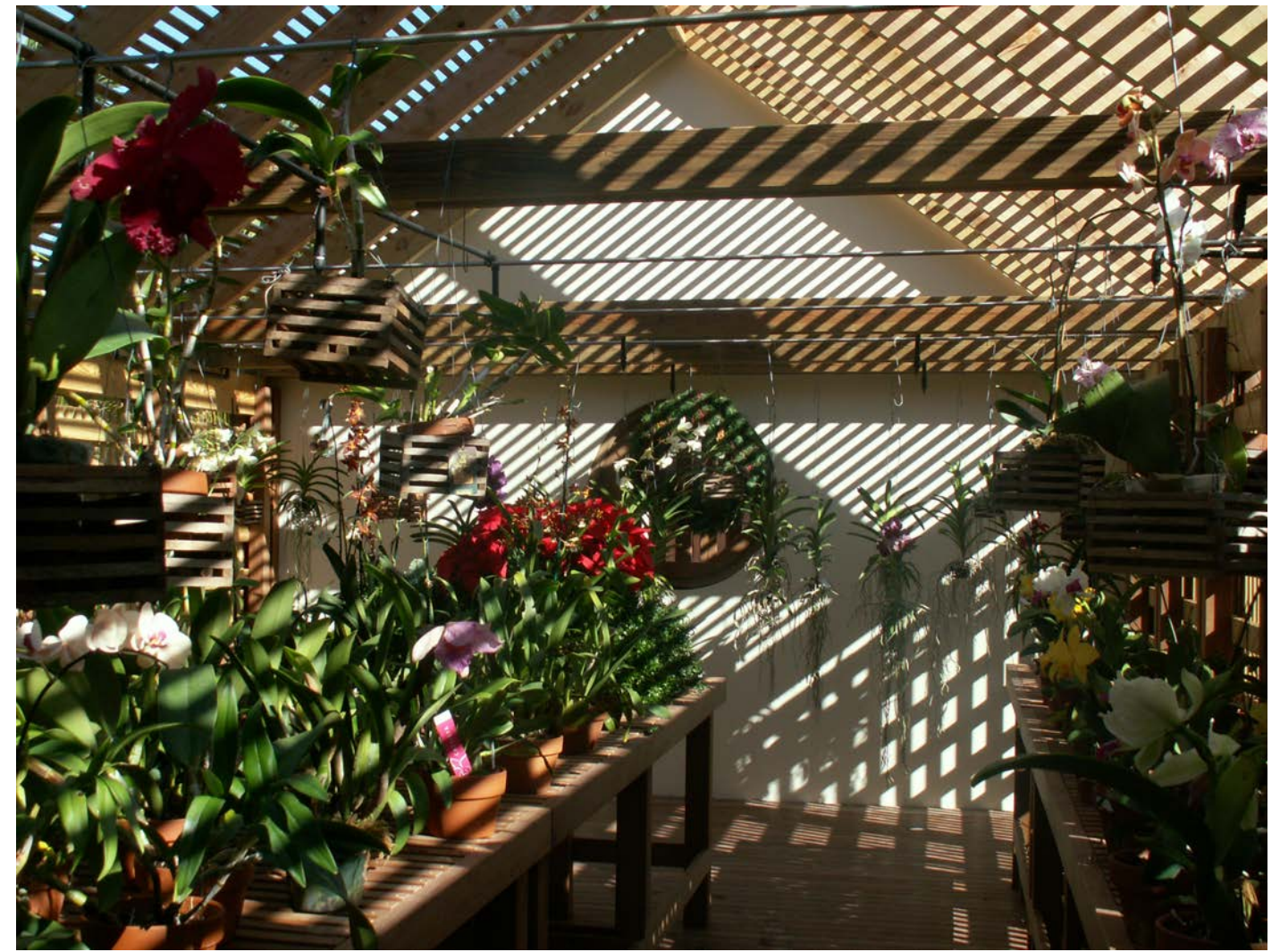
This orchid house in Jupiter Island, like the grapefruit sorter of the preceding page, and the interior of the Seaside Chapel, is a building type influenced by a tradition of agricultural buildings like corn cribs and grain elevators. Here an elevated wood floor between masonry end walls provides air circulation and the slatted walls and roof reduce direct sunlight.
